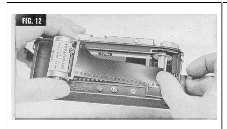
4. Holding right thumb on spool to prevent film pulling out, move film magazine to left end of camera and drop into its recess, allowing film to pay out from magazine as necessary. (See Figure 12.)
