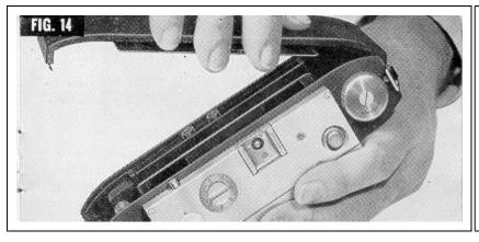
5. Replace camera back. in doing this, insert end with wide latch at left end of camera and swing closed as though it were hinged (Figure 14). Turn lock on bottom of camera to lock position.
