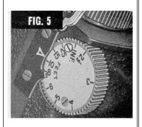
The coupled rangefinder of the REALIST makes accurate focusing quick and easy. Looking through the rangefinder eyepiece (right hand aperture at the bottom of the camera back) select any vertical line in the view and rotate the focusing knob (Figure 5) with the second finger of the right hand until this line in the upper part of the split field matches the line in the lower part of the field. See diagrams below.
