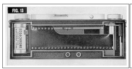
Figure 13 Shows film in proper position ready for winding (after camera back is replaced.) Note that edge of film is even with lower end of take-up spool so that entire bottom edge of film is parallel with bottom of camera.
