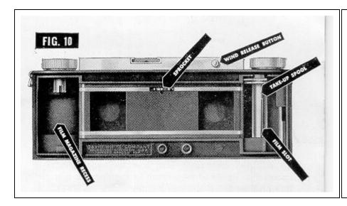
2. Return rewind release to normal position (2 dots together). Next, turn the sprocket (see Figure 10) in either direction with your fingers until it locks. Press film wind release button and turn winding knob until slot in film take-up spool is toward you. Pull rewind knob up as far as possible.
