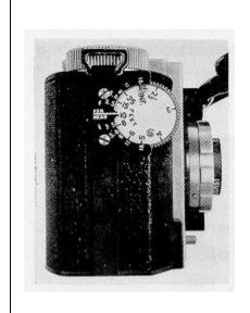
An important feature of your Stereo-REALIST. The Depth of Field Scale indicates the maximum range of sharpness, from the nearest point to the farthest point, that may be obtained with your REALIST camera for each particular picture taking condition.
