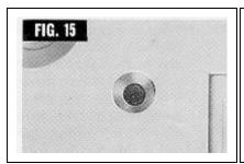
**9.** After each exposure, the shutter trip signal on top of camera (Figure 15) will show red. Repeat direction 7 to move unexposed film into position. After you have done this, the signal will show white indicating that the camera is ready for the next picture.
