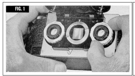
The iris diaphragm regulates the size of the opening which admits light to the camera. To set, rotate the rim of either lens to the required setting. (See figure 1.) Since the diaphragms of the two lenses are mechanically coupled this will automatically set both of them alike. information regarding proper diaphragm openings for various conditions is provided further on in this manual.
