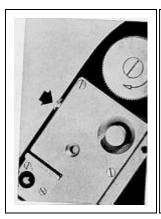
Leave double exposure button (indicated by arrow) in this position. With button pushed in you cannot fire shutter again until film is advanced.
