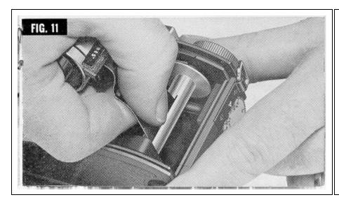
**3.** Holding film magazine in the left hand, insert 3. end of film firmly into slot in take-up spool. (See Figure 11.)
