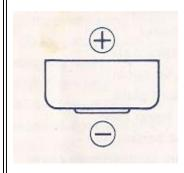
The battery will last approximately one year, depending upon the frequency of use. For replacement, we recommend the Eveready S-76 or equivalent. When you are not using the camera for an extended period of time, remove the battery.
