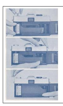
Do not load in bright light. Open back cover of camera by sliding back cover lock. Pull up the rewind crank knob, and put the film cartridge into the film chamber. Return the rewind crank to its former position. Draw out film leader and insert into take-up spool. If the slit is not in proper position to insert the film leader, turn the take-up spool.
