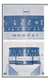
Infra-red rays focus slightly behind the film plane normally used for ordinary light rays. This, therefore, requires a modification of normal focusing procedures. First, focus in a normal manner. Then move the focusing ring from the index dot to the infra-red mark (15) on the depth-of-field scale ring.
