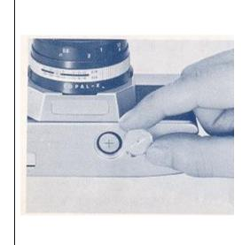
To open battery cover, use a coin in slot on base of camera body, turning it counter-clockwise. Then insert battery, with negative (-) side down.
