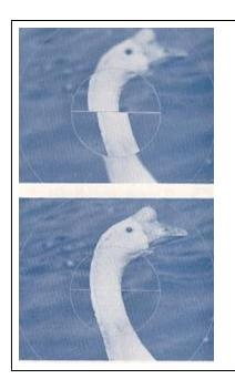
The rangefinder spot (split-image) located in the center of the viewfinder offers fast, critical focusing.
