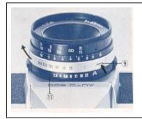
Set shutter speed ring on B (bulb) by depressing bulb setting lever (9). The shutter will remain open as long as the shutter release button is depressed, depending on the length of exposure desired.
