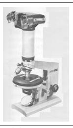
Photomicrography - yes, you can even take pictures through a microscope with your Zenith! At moderate magnifications no accessory is needed other than a rigid tripod or copy-stand to hold your camera, complete with lens, over the eyepiece of the microscope. For more professional results and and at higher magnifications the camera body should be attached direct to the microscope by means of a 42mm thread mount GA-3 Microscope Adaptor (obtainable through your dealer or direct from Zenith House).
