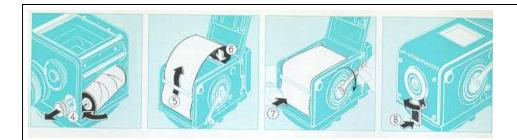
To open camera: turn the safety back lock clip at the tripod socket (I), lift back lock lever (a) and pull back open.
