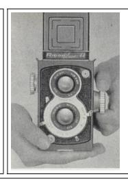
A Measure the proper exposure. Move the F stop and shutter speed selector levee and push down the shutter winding lever until it stops. After the shutter is wound the shutter winding lever returns to its former position. Therefore, whether the shutter is wound or not can be determined by moving the shutter winding lever. If the lever moves lightly then the shutter is wound.
