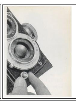
When using the self-timer, first wind the shutter, push down the self-timer lever. and release the shutter button. From the time the self-timer starts till the shutter is released takes about 10 seconds.
