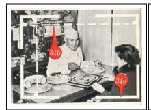
When you look correctly through the eyepiece of the finder, you will see a reflected line frame (34a). It outlines your picture area and is always plainly visible. This helps you to find the correct field of view and prevents faulty sighting. This is especially important with color shots, as you cannot easily trim a color transparency.
