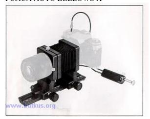
Designed for taking ultra-close-ups, it provides 1-3X magnification in combination with a 50mm normal lens. It is equipped with an automatic diaphragm to allow you to focus with the aperture wide open. Convenience accessories include a focusing rail and a slide copier.
