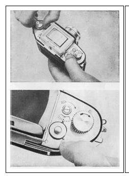
If, on the other hand, the film is wound into an empty cartridge instead of into the take-up spool, only 36 exposures can be made. As soon as the counter (15) points to "36", make two more "blind" exposures, so that all 36 exposed frames will disappear into the cartridge. Open camera back, take out feeder cartridge, open the latter and detach the film end from the center spool. This done, remove the take-up cartridge and wind up the rest of the film by turning the top of the center spool.
