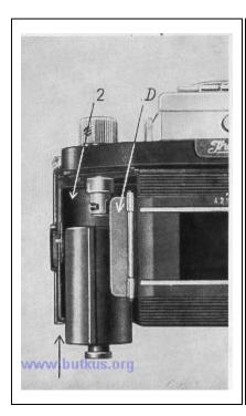
The EXA uses perforated miniature cine-film of 35 mm, width for 36 exposures  $1 \frac{1}{2} \times 1$  in. (=24x36 mm.) on a strip of the usual length of 1.60m. The film is supplied either in factory filled cartridges or an empty cartridge is loaded with refill film or with bulk film. For further details apply to your photo dealer. When using bulk film no special trimming of the film end is necessary except rounding off the angles.
