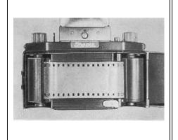
If there is no image visible in the finder-hood, wind film transport knob (4) up to the stop in the direction of the arrow. Release by pressing shutter release knob (27): first "blind" exposure. Wind knob (4) again up to the stop and release again: second "blind" exposure. (webmaster: these are the typical "blank" shots to move exposed film out of shutter area) Wind film transport knob a third time as far as it will go: an unexposed piece of film is brought into position in the image frame (8).
