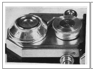
The indicator (exposure marker) is t triangle engraved on the lever (8). Pre shutter release button (9). Make two blank exposures by winding lever and pressing shutter release button The exposure counter will point to exposure No. 1, and the camera is ready for your first picture. You can be sure that the film transports in your camera properly if the rewind knob (3) turns counter clockwise as you turn the lever (8) to the right.
