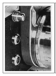
The EDIXA-Reflex is fully synchronized for regular flashbulbs and electronic flash. On
