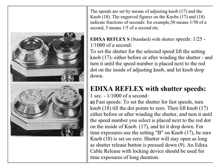
**b)** Slow Speeds: To set shutter for slow speeds lift Knob (17) and turn it until the speed "25" (1/25 of a second) is placed next to the red dot on the inside of Knob (17). Then turn Knob (18) to the selected speed, (for instance 1 second.)
