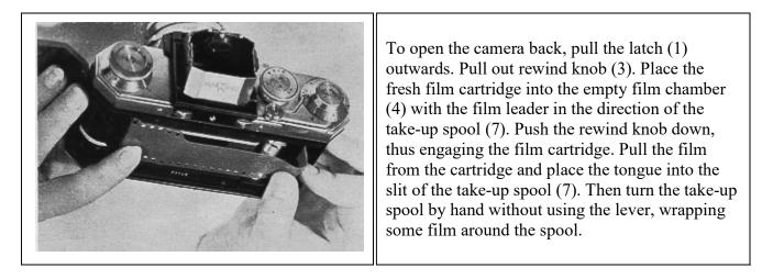
Be sure that the teeth on the sprocket wheel (6) engages both top and bottom rows of perforations on the film, before closing the camera back, and see that the film lies evenly on the film track (Close the back of the camera and pre latch down to secure. Turn lever fully, then set exposure counter (10) direction of arrow) on number 36.
