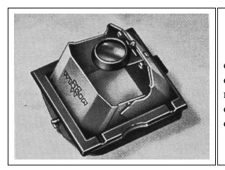
It will appear sharp. At the same time you are composing your picture, and controlling the depth of field. For critical focusing, use the magnifier, keeping it close to your eye. Before closing hood, be sure to fold the magnifier down.
