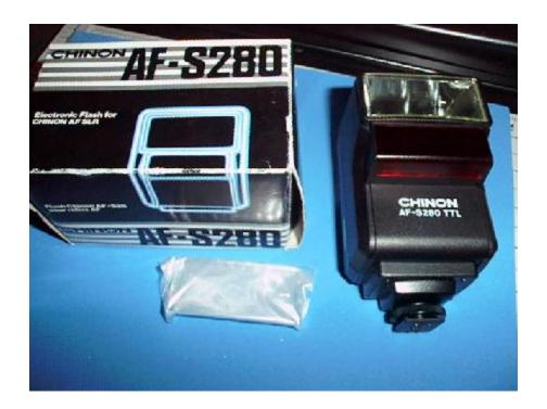
This flash provides AF and "Through The Lens Flash" with the Chinon CP-9AF camera other flashes will require you to go to manual mode and manually set the camera's aperature — the small white item is the wide angle flash adaptor —
