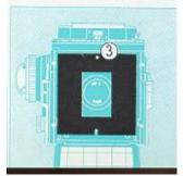
Adjusting the film pressure plate ( --> page 9): slide plate downward until inscription 1 x 1 1/2" (24 x 36 mm) is visible.
