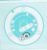
Loosen both screws on the front of the meter (I), until it can be removed from the focusing knob.
