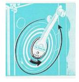
The correct diaphragm opening is indicated in the center of the peep window. Intermediate values can be used (f/3.5 is a midpoint stop between f/2.8 and f/4 in the international diaphragm scale).
