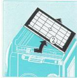
To lift the focusing screen: take hold of the two sides of the frame, pull backwards slightly and lift (2) Close by pushing downward.
