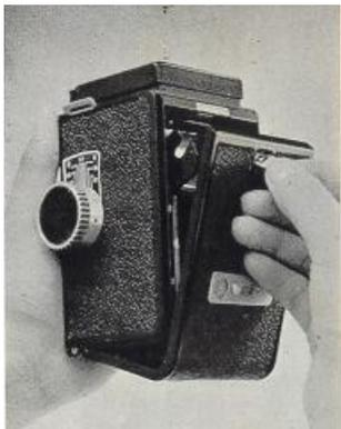
1. Raise the back cover locking tab and turn it counter-clockwise to open the back cover.
