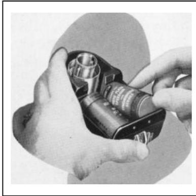
The front part of the battery case is removable. Hold the unit in the left hand and pull off cover with right hand.
