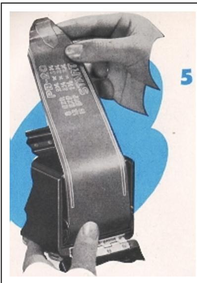
Holding cradle in with the left hand, pull off about 8 inches of paper leader for threading.
