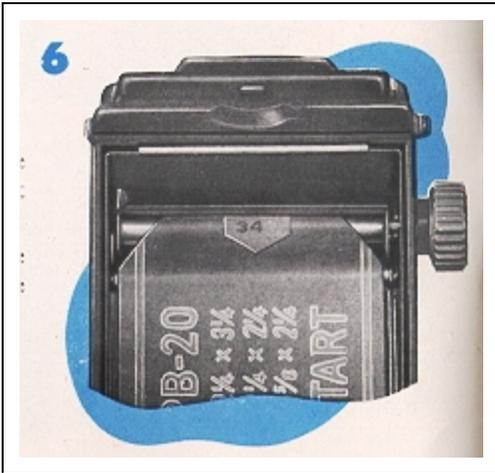
Fold end of paper (about one inch) and insert into long slot of the empty film spool. To secure end of paper, give the winding knob about three turns.
