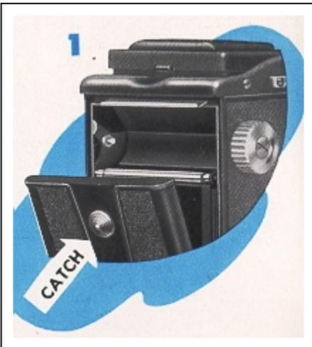
Open the back of the camera by pressing down on the locking catch. The back is hinged for convenience. Hold camera so back does not drop or hinge may be sprung.
