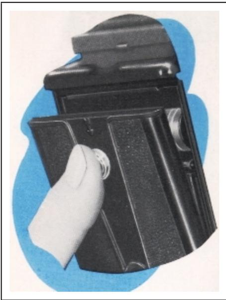
Open the back of the camera by pressing down on the locking catch.
