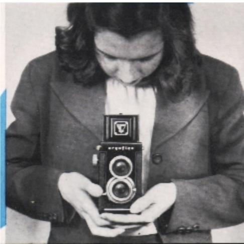
To take the picture, hold the camera as shown, and compose the subject on the ground glass as you want it to appear in the finished picture. A lower or higher position may be desirable to get just the effect you want. Then, hold your breath for an instant and press the shutter release SMOOTHLY with the right thumb. Take care not to jar the camera or the picture may be blurred due to camera movement.
