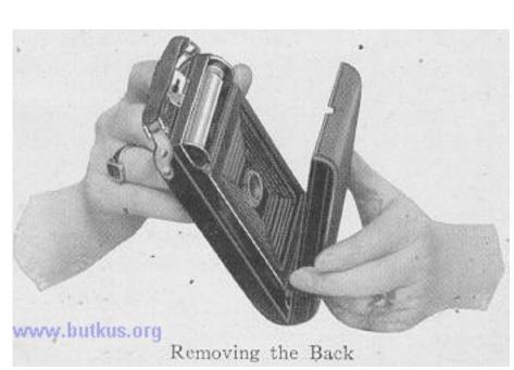
Open the back of the camera by releasing the hinged catch at one end and removing the metal back, so as to have access to the spool chambers.
