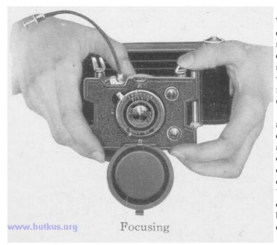
The ANSCO V-P No. 2 is equipped with a micrometer focusing device consisting of a milled disk and flange which permits accurate focusing for distances of 6, 8, 10, 15, 25, 50 and 100 feet. A small window at the top of the camera contains the focusing scale and pointer. The figures on the scale indicate the distance in feet. If it is desired to use an ANSCO V-P No. 2 as a fixed focus camera, the scale should be set at 25 feet and the diaphragm at F 11, or F 16.
